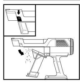
To empty the handheld vacuum (IW3600ANZ Series) dust cup, turn off the power and hold the hand vac over the trash. Press the release button and the dust cup lid will drop open. releasing debris.
