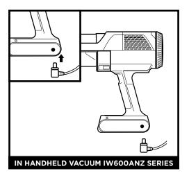
To charge the battery inside the handheld vacuum, insert the charger into the port below the handle on the handheld vacuum, then plug the charger into an electrical outlet.
