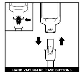
To detach the hand vacuum from the wand. press the front latch release button on the hand vac where it meets the wand, then lift off the hand vacuum. To reattach the hand vacuum to the wand, align the hand vacuum opening over the top of the wand and slide it on until it clicks into place.
