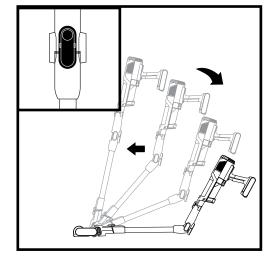
Press the unlock latch on the back of the wand, then adjust the angle.
