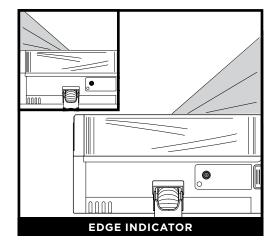
When an edge is detected, the headlights will illuminate on one side where the edge is detected, to focus on targeted debris.
