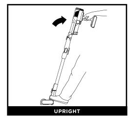
When upright, the nozzle will lock to allow for free standing storage when the hand vac is detached. Place your foot on the nozzle to disengage the lock to begin floor cleaning.
