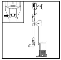
Place the vacuum on the dock in a downward motion. Once properly attached, the auto evacuation process will begin. The evacuation cycle will last for 15 seconds.
