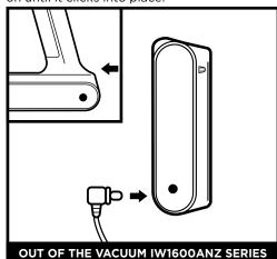
Press and hold the Battery Release Button. then pull out the battery. Plug the charger into the charging port on the battery. To reinstall the battery, insert it into the slot in the back of the handheld vacuum.
