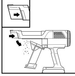
To empty the handheld vacuum (IW1600ANZ Series) dust cup, turn off the power and hold the hand vac over the trash. Press the release button and the dust cup lid will drop open, releasing debris.
