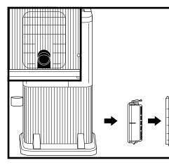
To access the filter in the dock, remove the Filter Door. Press the button at the bottom of the door, then tilt the door and lift it off. Remove the filter from the dock. After the filter has been rinsed and dried, reinstall it by reinserting it into the dock and replacing the filter door.
