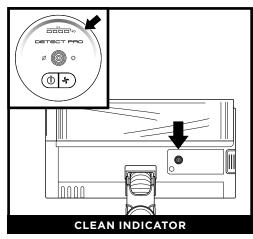
When the LED Indicator light is blue, this means no heavy debris is detected and suction power is normal. When the vacuum senses heavy debris, the light will turn red, and suction will increase for more cleaning power. When the indicator light turns amber, debrisis being removed—continue cleaning until the indicator turns blue again.
