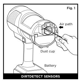
Make sure to clean the Detect sensors regularly, as hair and other debris may build up and obstruct them. If the sensors are partially obstructed, Auto mode will not function as expected.
