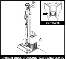
Charge the unit by placing it on the dock. Make sure the contacts on the wand are aligned with the contacts on the charging post. When charging is complete and you need to use the unit again, lift it off the dock.
