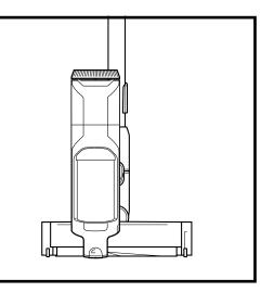
For quick and easy short-term storage, attach the hand vacuum to the wand by placing it onto the pre-assembled wand storage clip.
