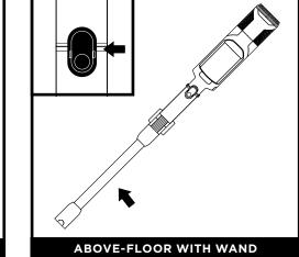
To detach the floor nozzle from the wand, step on the nozzle while pressing the nozzle release button at the bottom of the wand. Lift the wand to remove it. To reattach the wand, align it over the neck of the floor nozzle, then slide it on until it clicks into place.
