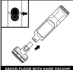
Detach the hand vacuum to clean abovefloor areas. Press the front latch release button on the hand vac where it meets the wand, then lift off the hand vacuum. To attach an accessory to the hand vacuum, slide it into the opening in the nozzle. To remove, press the front latch release button on the hand vac where it meets the wand, and slide out the accessory.
