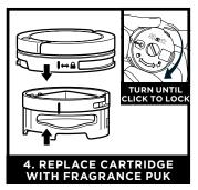
Align the yellow arrow on the side of the fragrance puk with the yellow arrow on the side of the Odour Neutraliser Technology Dial cover, then insert the fragrance puk into the dial. Rotate clockwise to lock it in place.
