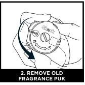
Rotate the fragrance puk anticlockwise in the Odour Neutraliser Technology Dial housing and pull out the fragrance puk to remove it.
