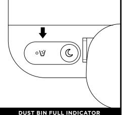
The Dust Bin Full indicator will illuminate when the dust bin is full of debris and needs to be emptied. To reset the indicator, remove the dust bin and empty it.
