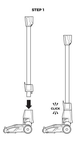
1 Insert the wand into the motorised floor nozzle connector until it clicks into place.
