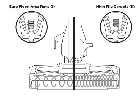
The Shark® Rocket™ Complete with DuoClean® has a 2-speed power slider switch on the handle. Slide the power switch to appropriate speed setting (I or II) and start cleaning.
