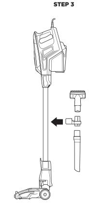
**3** This vacuum comes with a detachable clip to store up to 2 accessories on board. Snap clip onto the wand. Store one accessory on top holder and one accessory on bottom holder.
