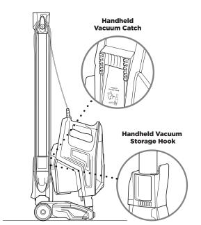
1 Press the Wand Release button at the top of the wand to detach the handheld vacuum. Align the catch on the bottom of the handheld vacuum with the storage hook on the wand. Slide the handheld vacuum down so the catch hangs from the storage hook. Wrap the power cord around the top hook first, leaving a little slack while wrapping.
