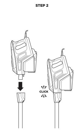
2 Insert the handheld vacuum into the top of the wand until it clicks into place.
