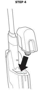
**4** To replace the water tank, align it so the cap faces down. Place the cap into the hole in the Steam Mop body and slide tank down until it clicks securely into place.
