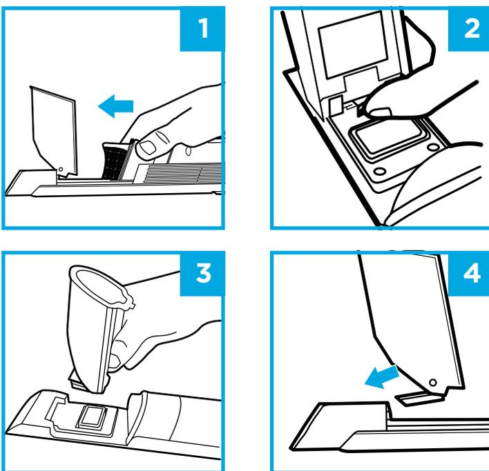
1. With the dust cup open and the power off, pinch both sides of the filter housing and slide it forward to remove.
