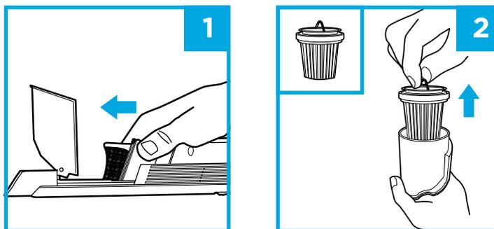
1. With the dust cup open and the power off, pinch both sides of the filter housing and slide it forward to remove.
