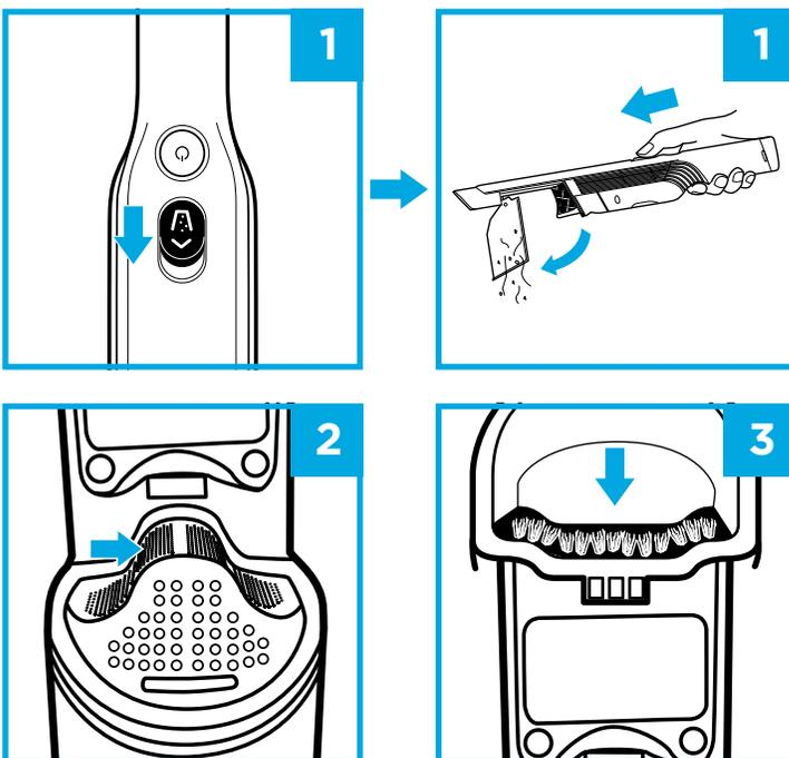
1. With the power off, slide the Open Dust Cup button forward, and the dust cup will swing open.
