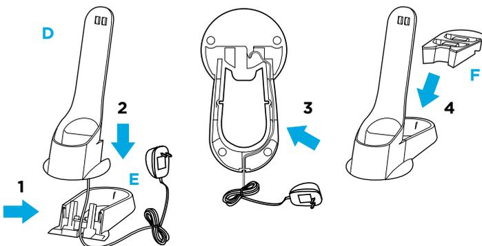
1. Align the holes in the bottom of the **ION Charging Stand** with the posts on the front of the **Charging Base**. Run the **Charger Cord** through the groove.
