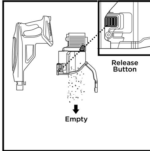
To remove the dust cup from the handheld vacuum, squeeze the two **Dust Cup Release** buttons at the same time and pull out the dust cup.
