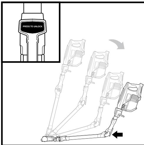
Press the unlock latch on the back of the wand, then adjust the angle.
