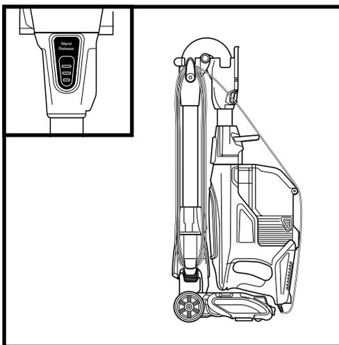
Looking at the vacuum from the side with the cord hooks, wrap the power cord anti-clockwise around the hooks, starting under the bottom hook. Then press the **MultiFLEX Wand Lock Release** button and gently fold the handheld vacuum forward toward the floor nozzle. Use the handle to carry the vacuum to its storage location.
