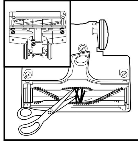
If you notice any hair wrap, continue vacuuming and the **Self-Cleaning Brushroll** will automatically remove it. If some hair wrap remains after continued use, remove the brushroll cover from the bottom of the nozzle and use scissors to carefully cut away the hair.
